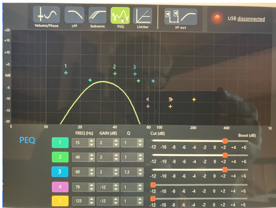
Figure 3: SPA500DSP Amplifier Default Settings
