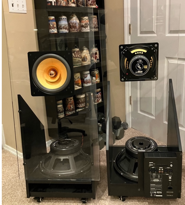
Figure 1: VPE Crystal Dipole Woofer Front and Rear Views
